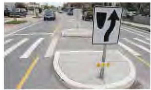
RAISED MEDIAN ISLAND Provides buffer and protection for pedestrians while crossing wide or busy streets. Adds space for green infrastructure. PHOTO: pedbikeimages.org/Dan Burden
